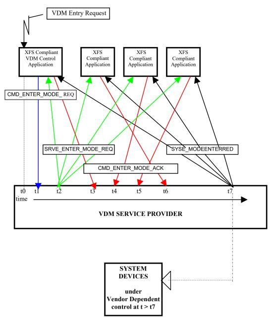
At time t0, status is "Inactive" and a request to Enter VDM arises from within the Application system. At time t1, an Application Process/Thread/Function issues the CMD\_ENTER\_MODE\_REQ Execute cmd. Status then becomes "Enter Pending".
